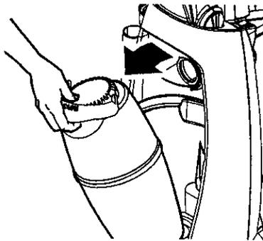
Remove dust bin from vacuum cleaner by tilting out as shown.
